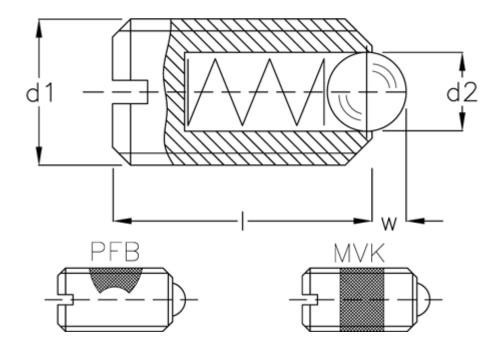
$\begin{array}{ll} \text{d1} & = \text{M12} \\ \text{d2} & = 8.0 \\ \text{Length I} & = 22 \\ \text{Spring pressure N bottom} = 49.0 \\ \text{Spring pressure N top} & = 26 \\ \text{W} & = 2.5 \end{array}$
